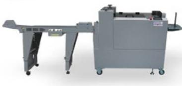
Separator and conveyor units remove skeleton/waste portions
